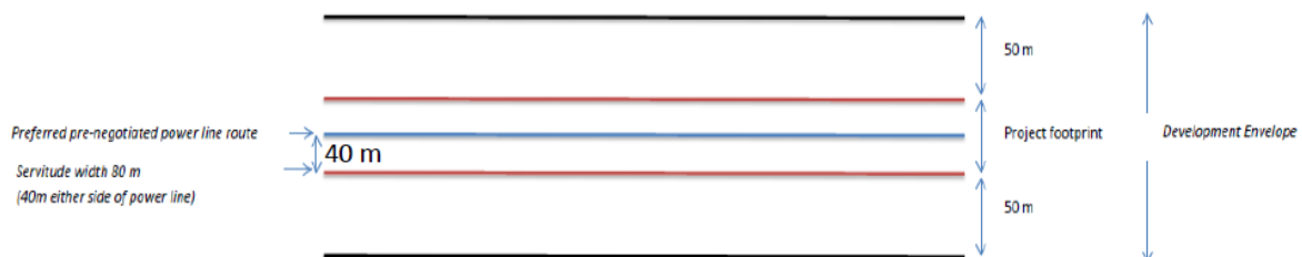
Figure 1: Diagram of the typical footprint of a 765 kV powerline corridor (DEA, 2016).
