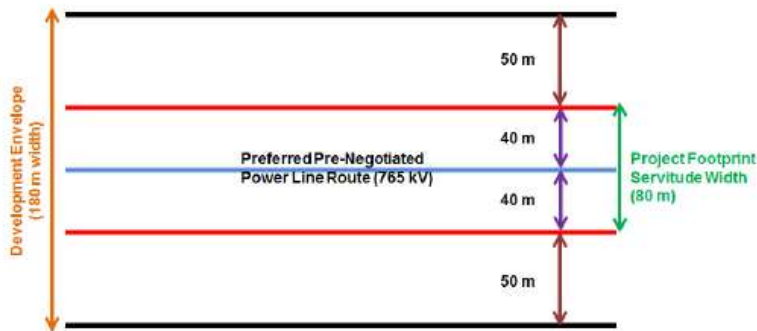
Figure 1: Route Profile: Servitude and Development Envelope for a typical 765 kV power line (DEA, 2016)
